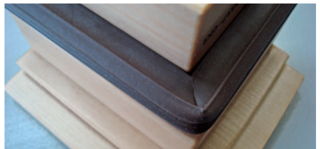
Richtige Position Correct position of corner cut
